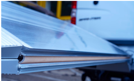
Even force distribution across the platform thanks to the belt hinge.
