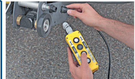
Emergency control by cable remote control.
