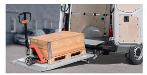
When unfolded, the large platform provides sufficient space to load and unload one pallet with a forklift and up to four trolleys. A platform height of 72,05" (1830 mm) and a carrier vehicle with a high roof are required for transporting pallets with forklifts.
