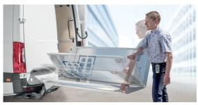
For large quantities, the platform is opened hydraulically with the Bär SmartControl remote control and unfolded manually.
