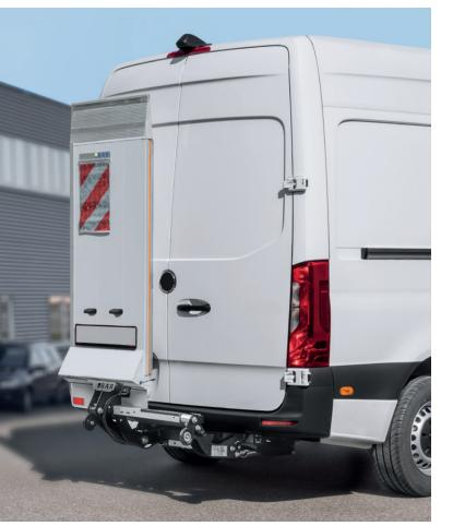
If you require free access to the cargo space, but also require the ability to load or unload pallets or trolleys at any time, the Bär FreeAccess VanLift offers you unimagined freedom when using your panel cargo van. The minimal weight, quick fitment, usually without chassis work, and trailer operation still set standards in the VanLift class years after its market introduction.
