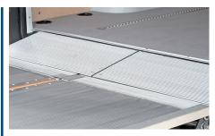
Connecting platform and panel van while allowing free entry through the right rear door: **Bär VanBridge**.
